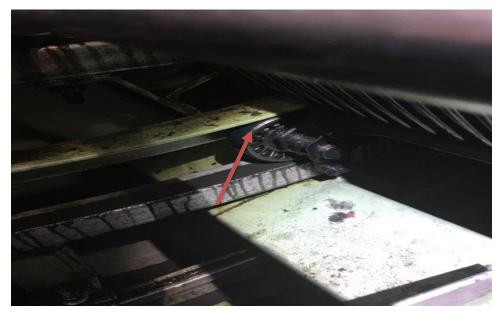
Example of a properly adjusted upthrust track, showing the correct clearance.
