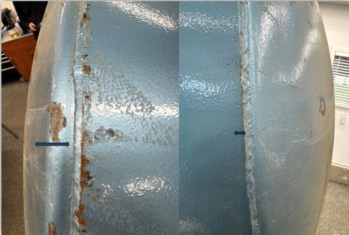
Image 20 - Upper head of Supply Tank 2 after failure. Note difference in distance between the circumferential weld and the break in the head, from left side to right side. Tank constructed outside of code requirements for margin of error.
