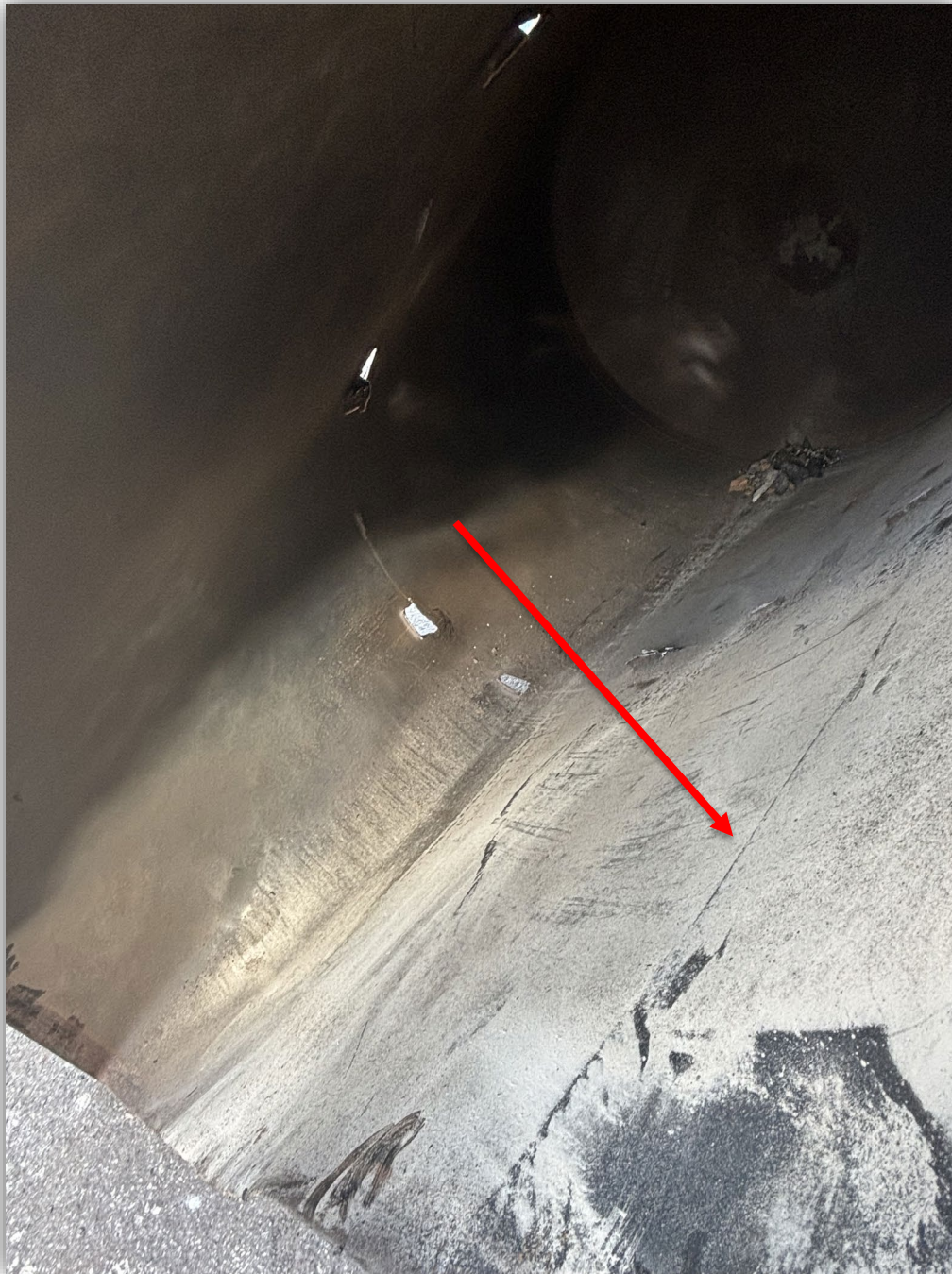
Image 17 - Inside of Supply Tank 2. Longitudinal weld seam indicates zero penetration and no welding from the inside of the vessel.
