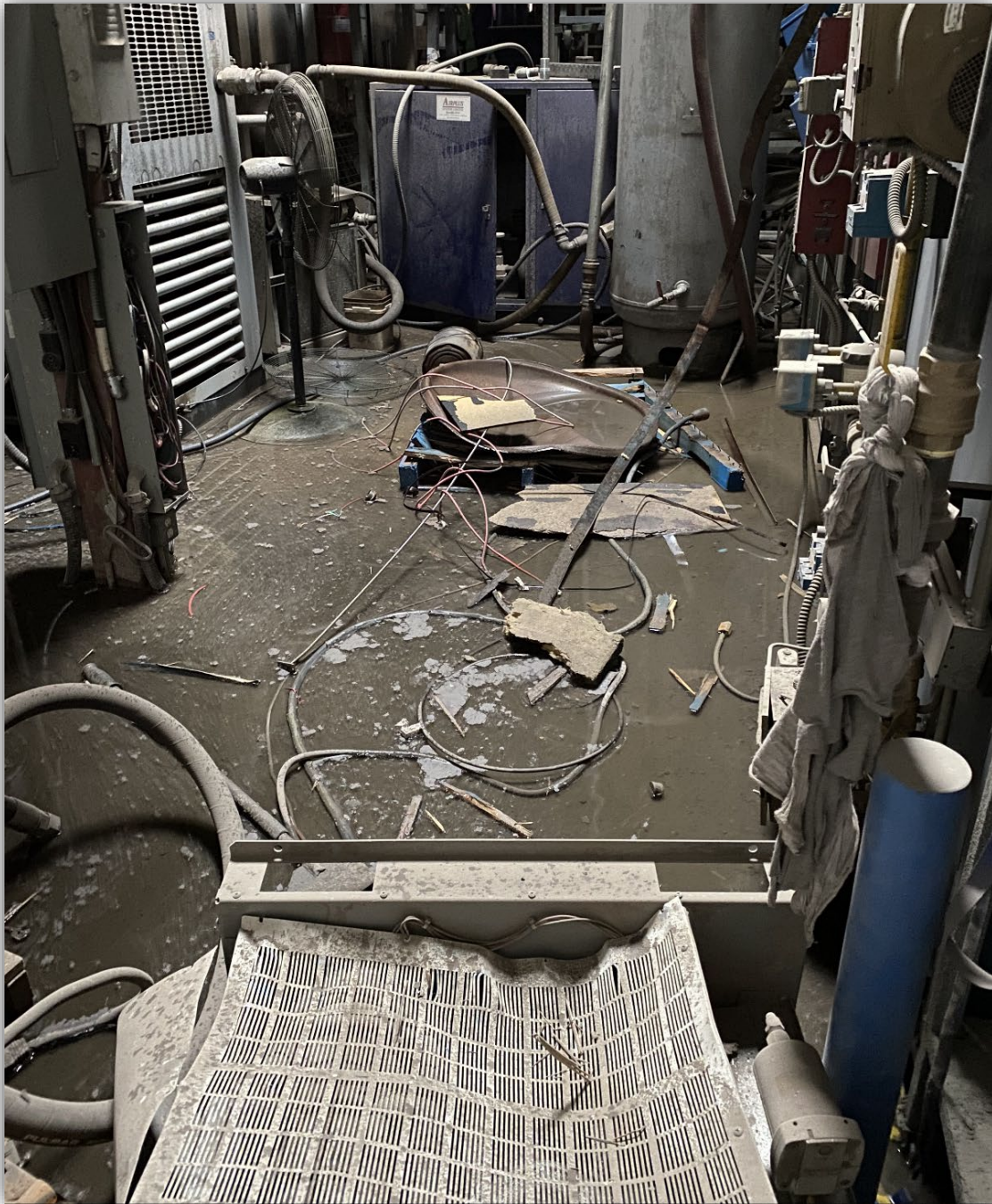
Image 4 - Supply Tank 1 and remains of Supply Tank 2. Manager was kneeling on other side of Supply Tank 1 during incident.
