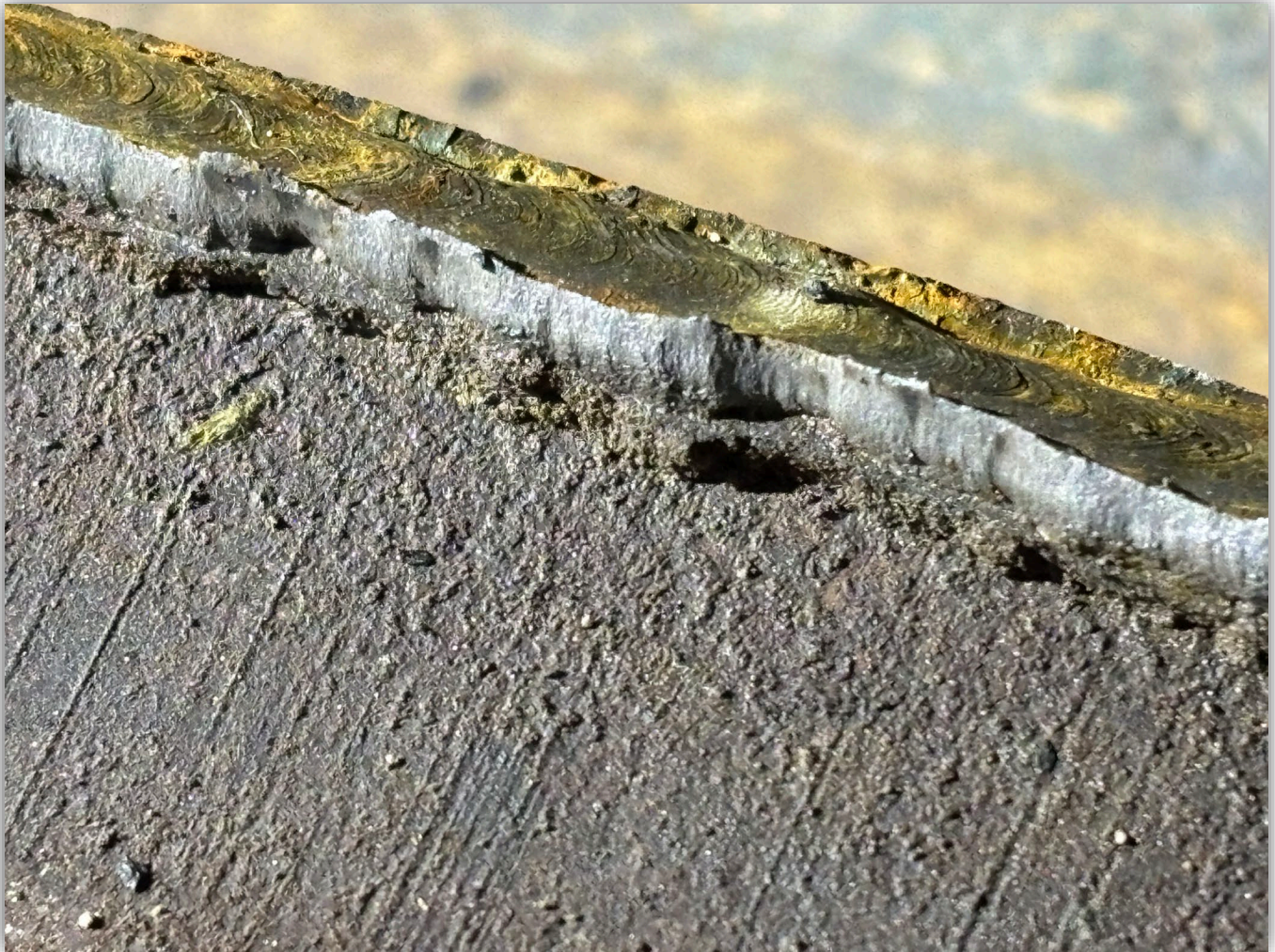
Image 15 - Close up of failed weld on inside of bottom head of Supply Tank 2.
