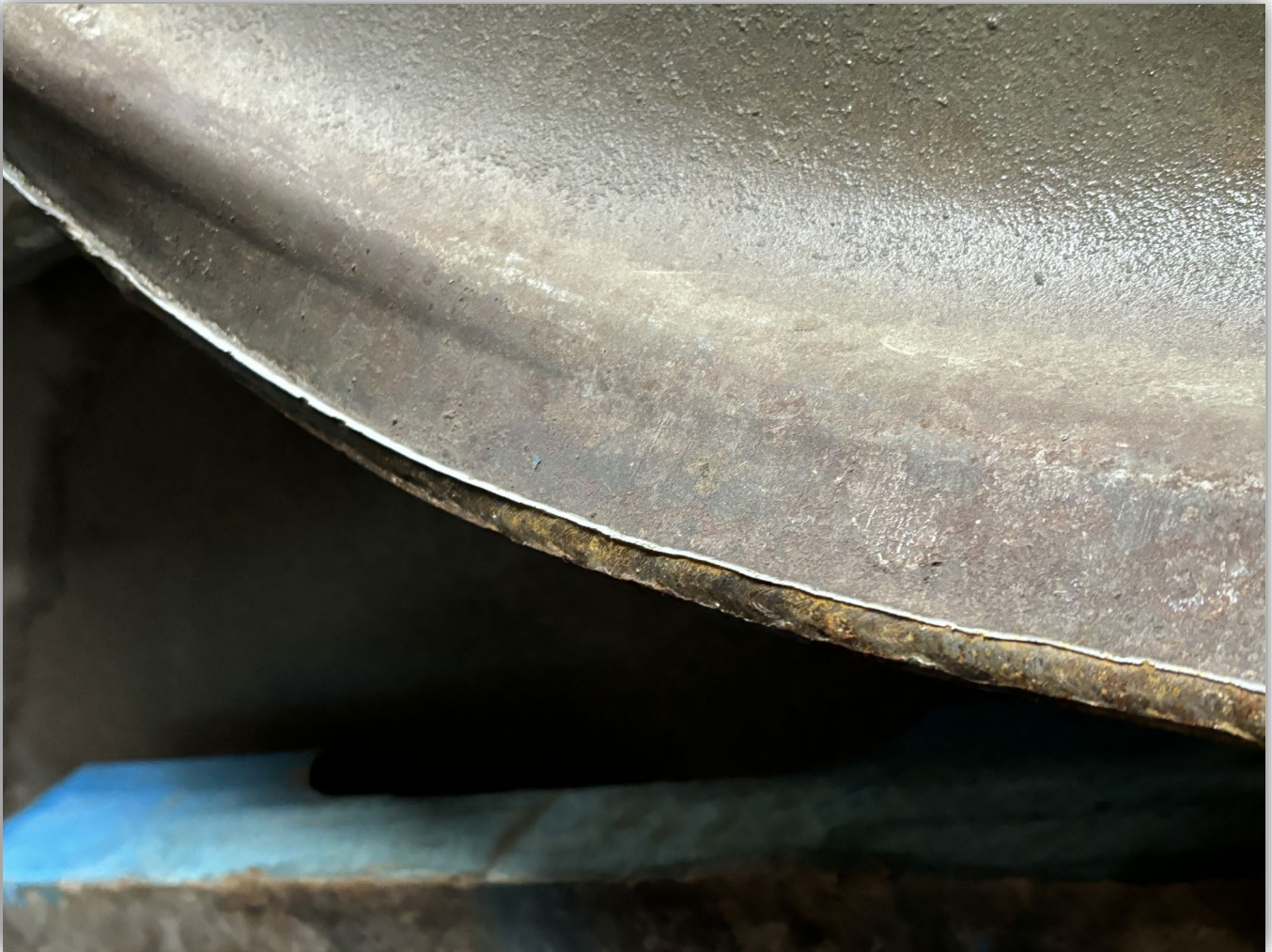
Image 14 - Failed weld on inside of bottom head of Supply Tank 2.
