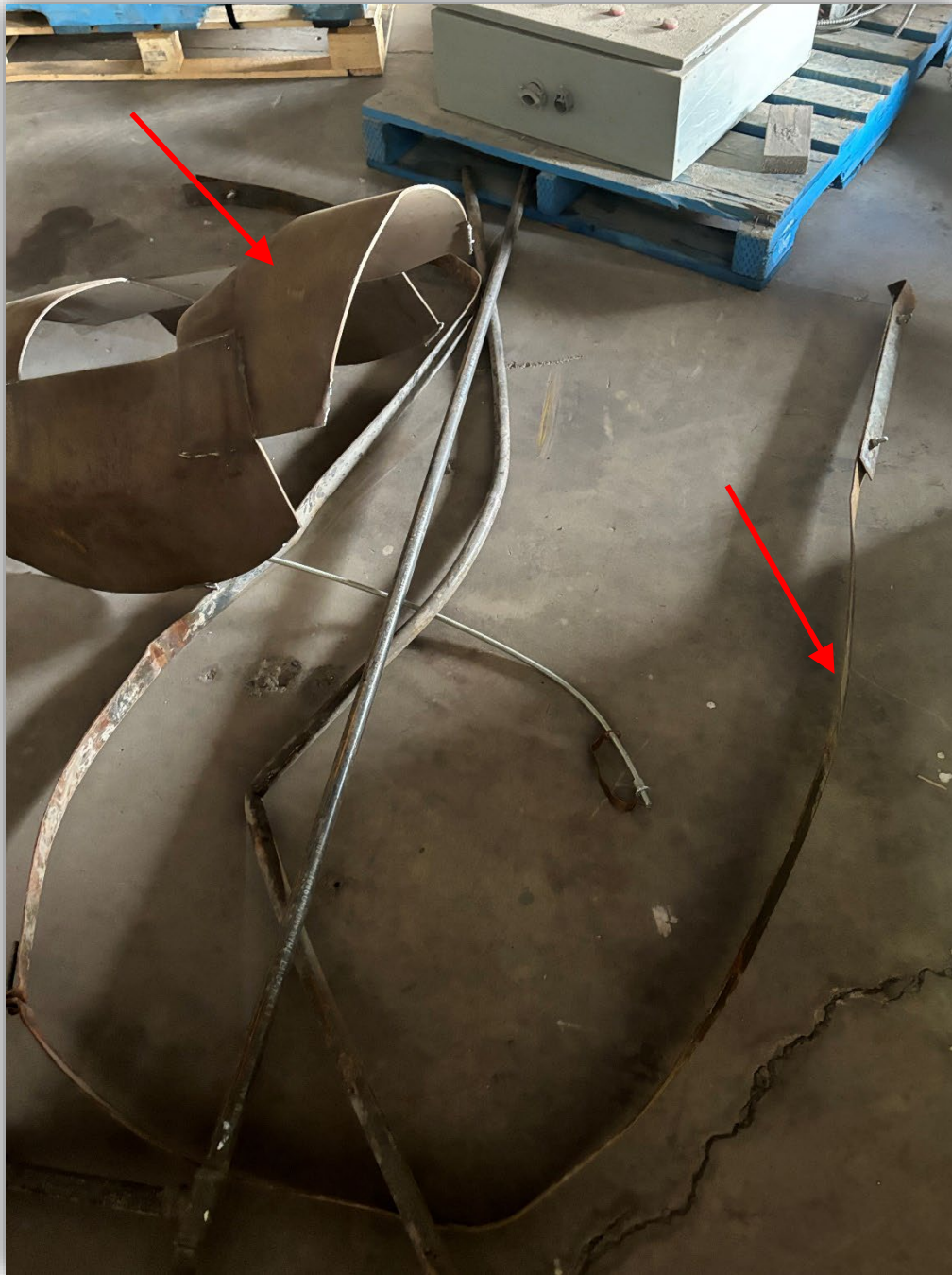
Image 11 - Internal baffle that was blown out of tank, and strap used to secure tank to pallet.
