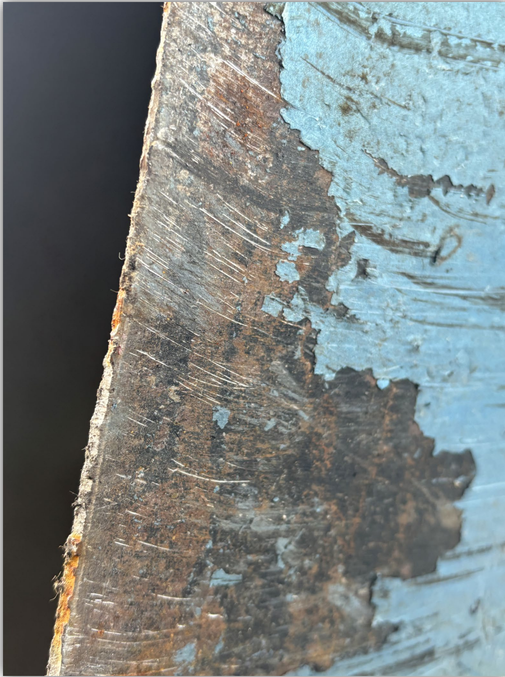
Image 16 - Failed weld on outside of shell of Supply Tank 2.
