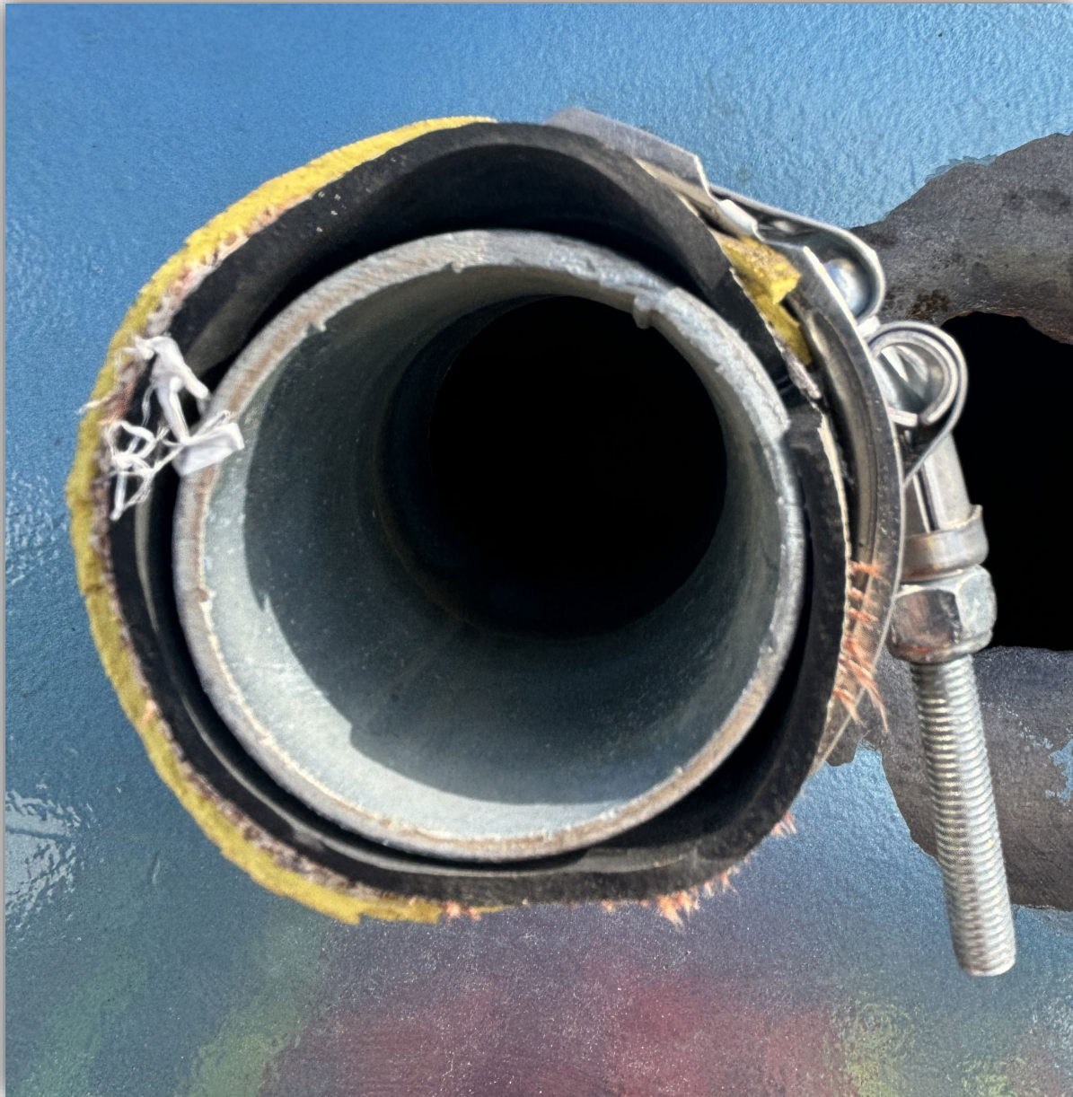
Image 12 - 300 PSI contractor grade 3" flexible airline, torn at attachment point.
