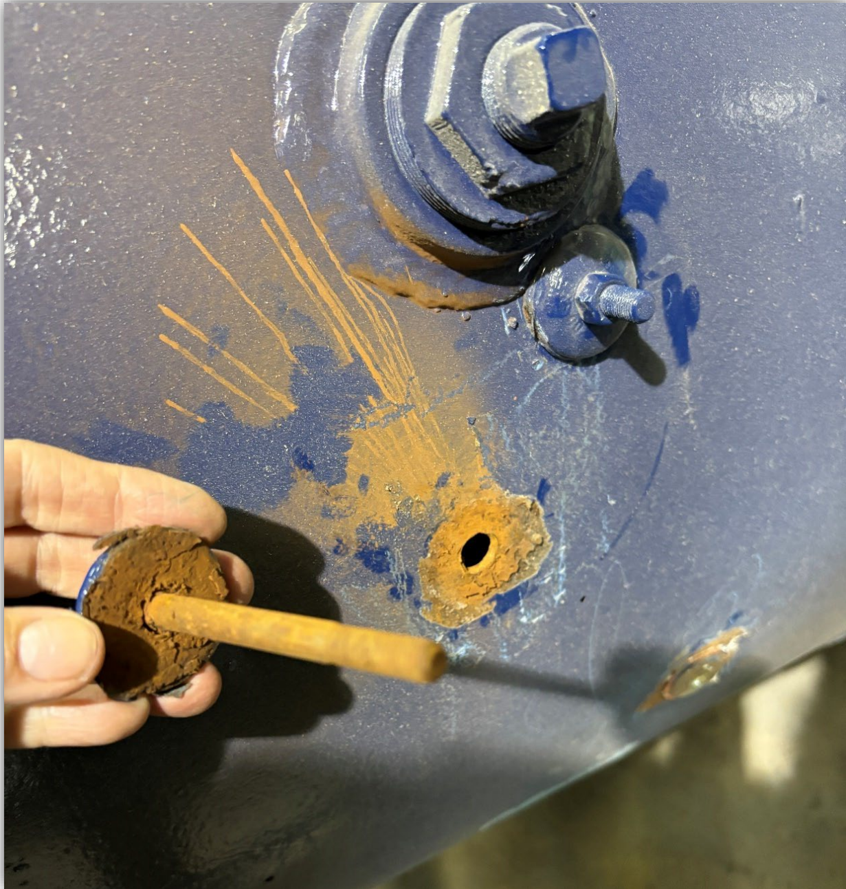
Image 24 - Supply Tank 3: owner discovered that three 3/8" decommissioning holes had been drilled in the tank in the past, then filled and hidden by inserting a bolt and washer and affixing with silicon.
