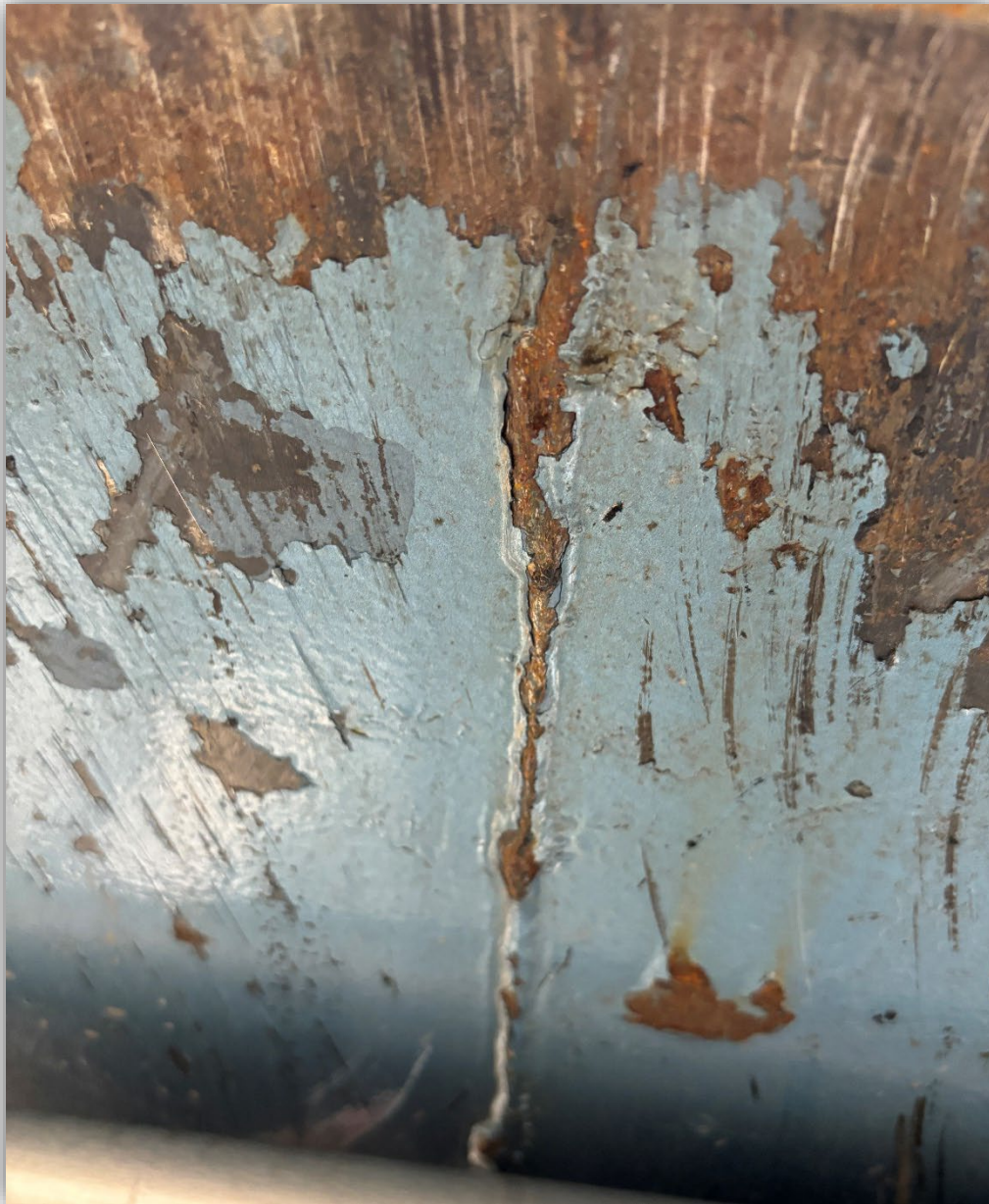
Image 14 - External weld of longitudinal seam.
