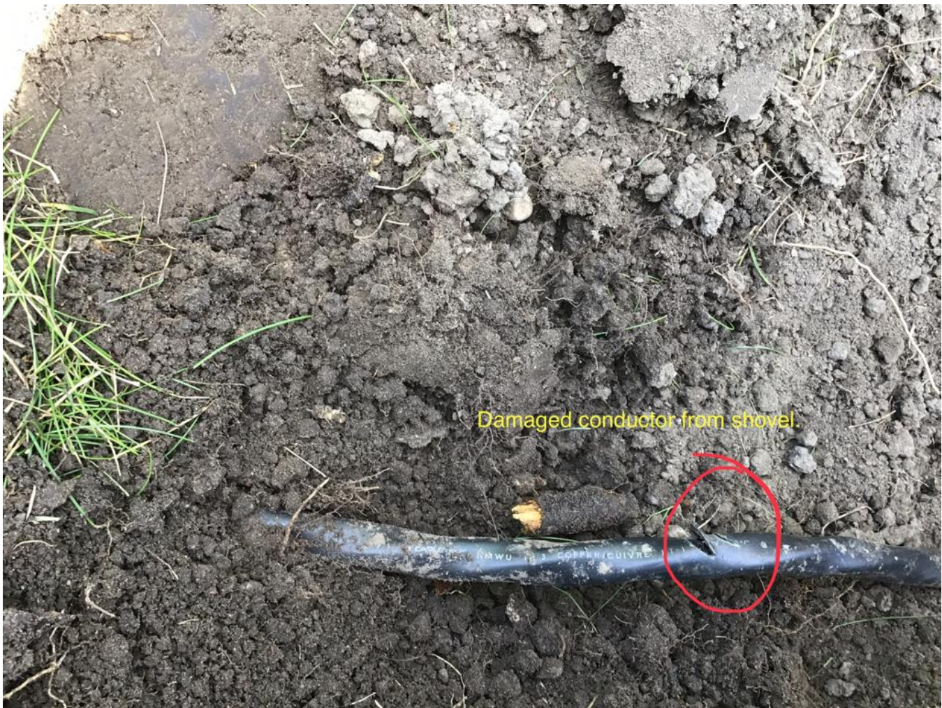
Damage to Direct Buried wire from shovel head
