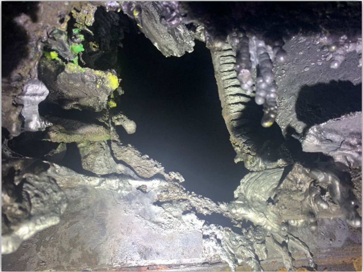
Image 2 – Melted hole in hearth burner wind box.
