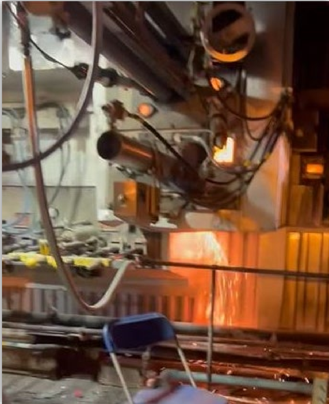
Image 1 - Flames exiting hearth burner wind box through melted hole.
