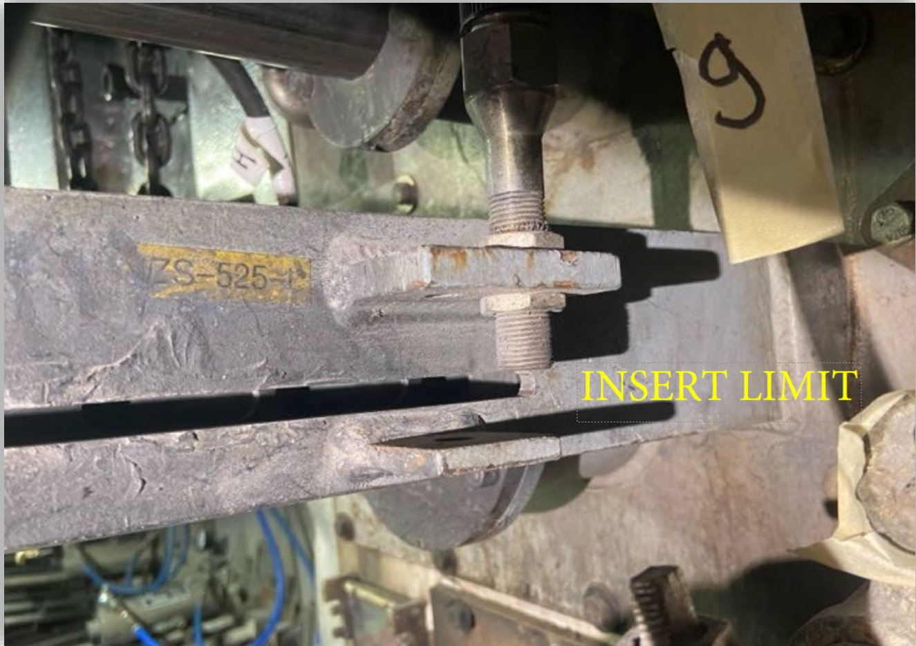
Image 5 – Limit switch without shims.
