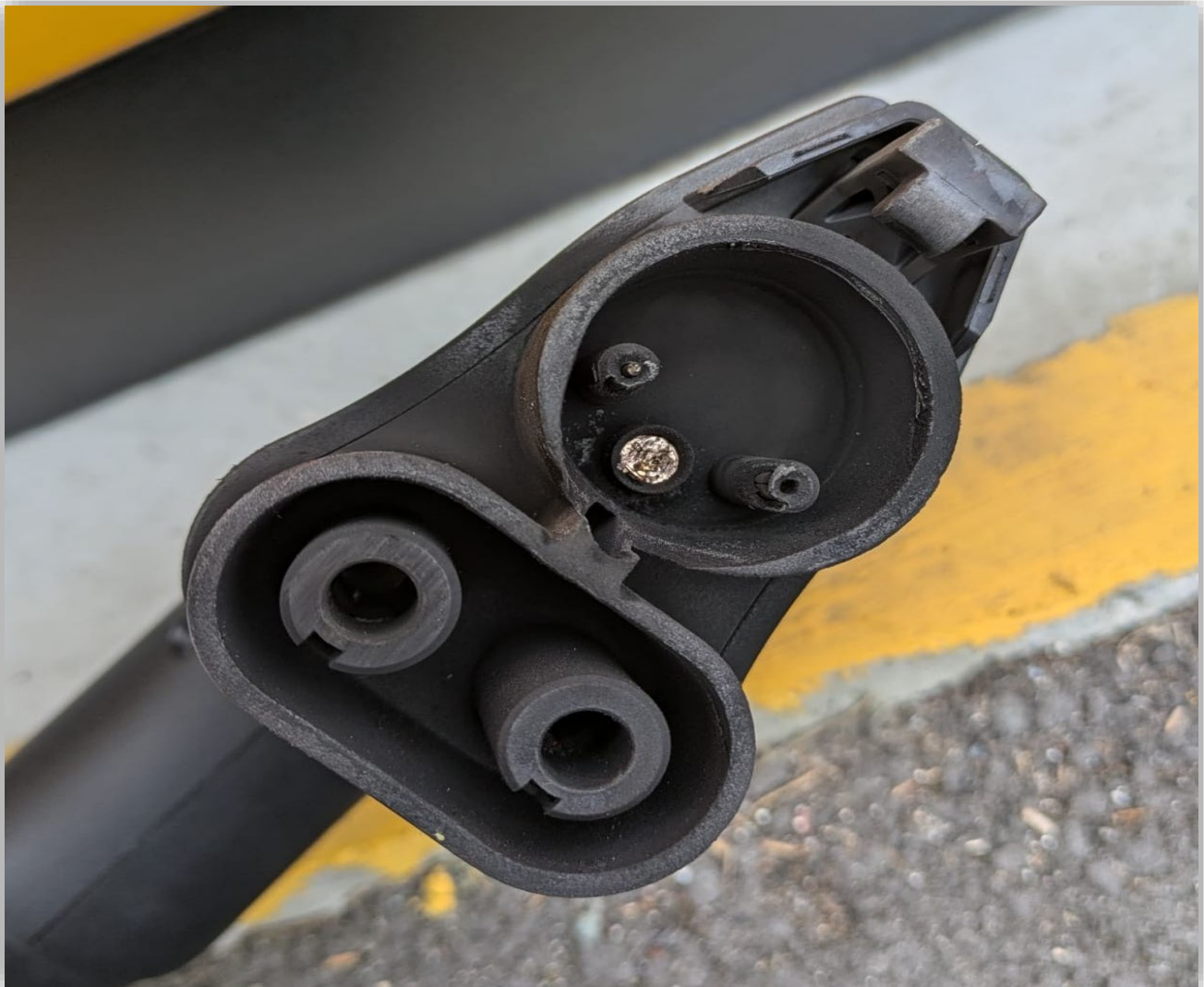
Image 3 - The ground terminal on the charging cable melted away.
