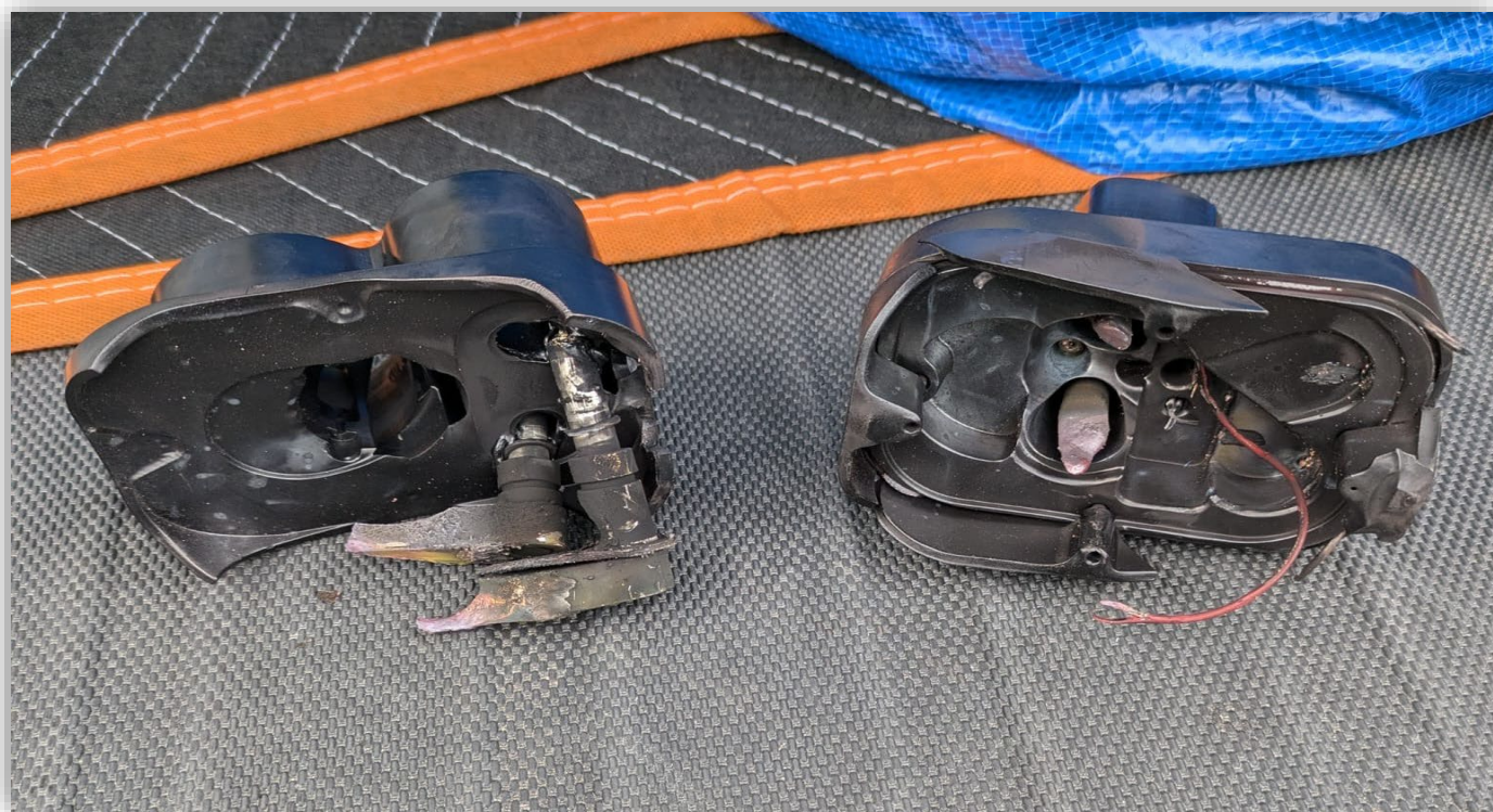
Image 2 - Adaptor blown in half with terminals showing signs of extreme heat.
