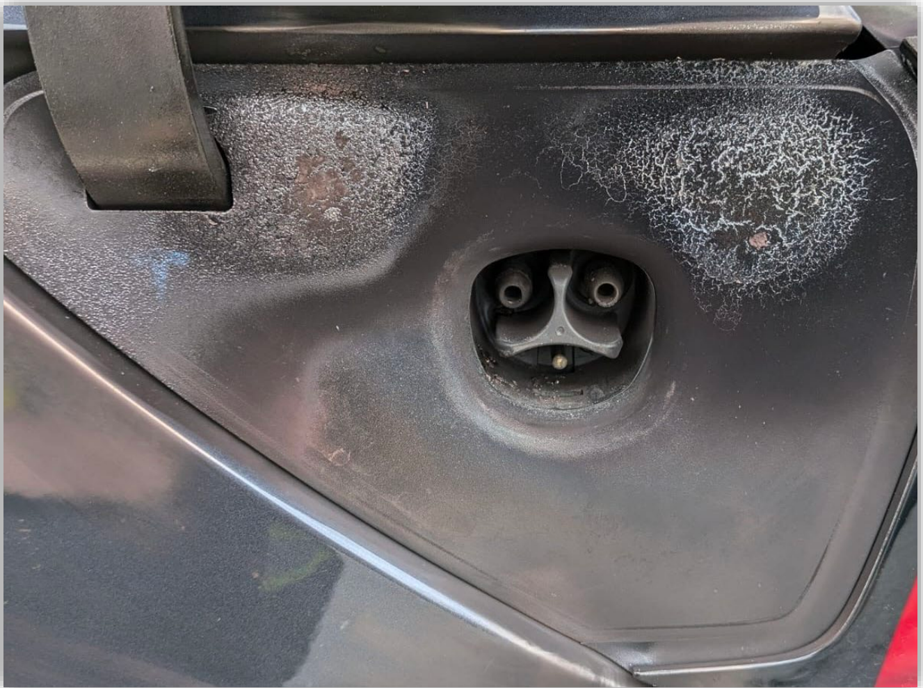
Image 4 - Electrical burn marks on the vehicle but charging terminals show little sign of damage.
