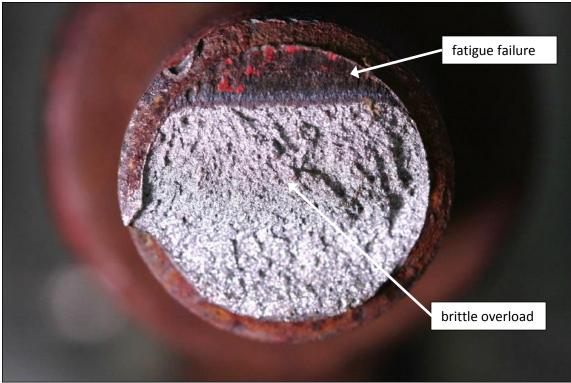
**Figure 6:** Fractured Surface of Eyebolt Threaded Shaft. (Photo, material and fracture surface analysis conducted by Acuren Group Inc – Richmond).
