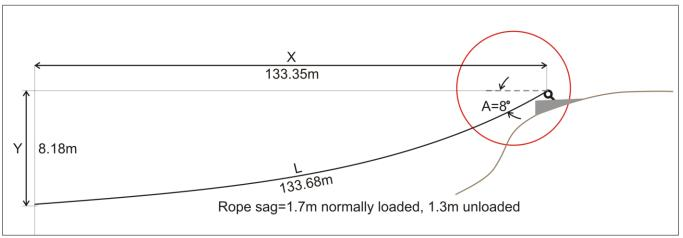
Figure 3: Profile of Zipline as Measured Following Incident
