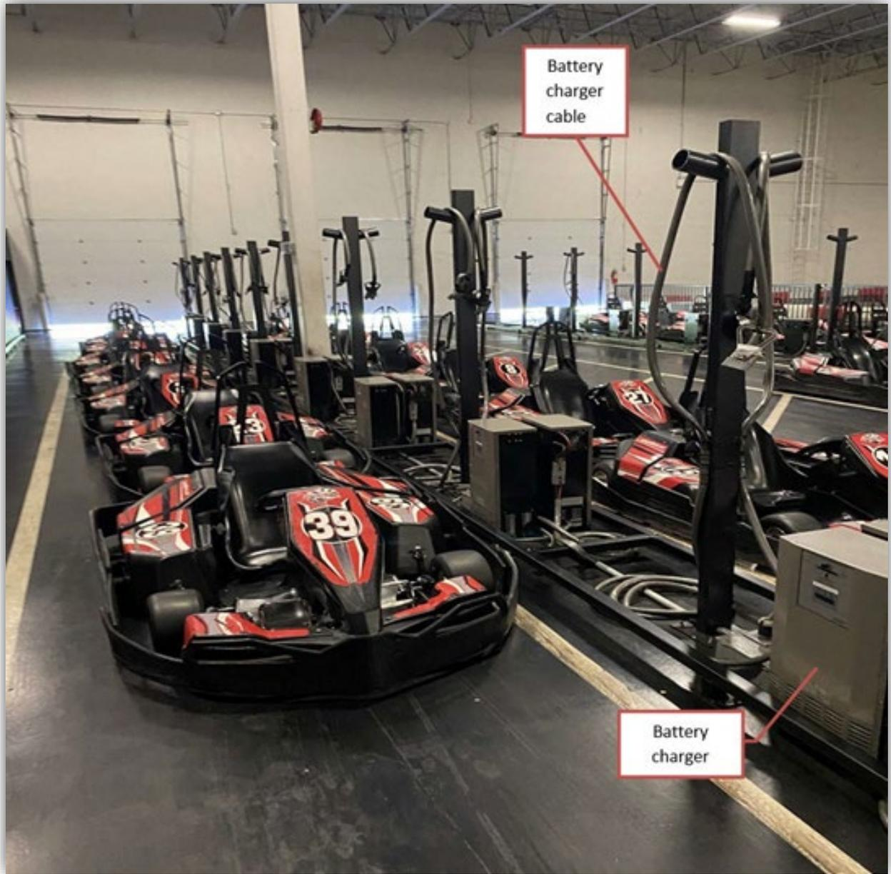
Image 1 - Go-karts ready to be charged. Battery chargers and battery charger cables are visible.
