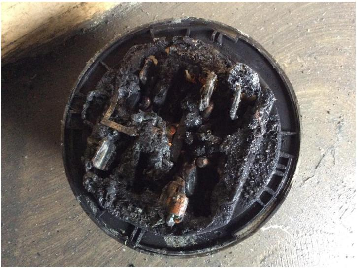
Rear of revenue meter showing damage radiating out from centre.
