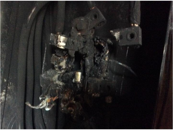
Inside of meter base. Showing damage radiating out from centre.
