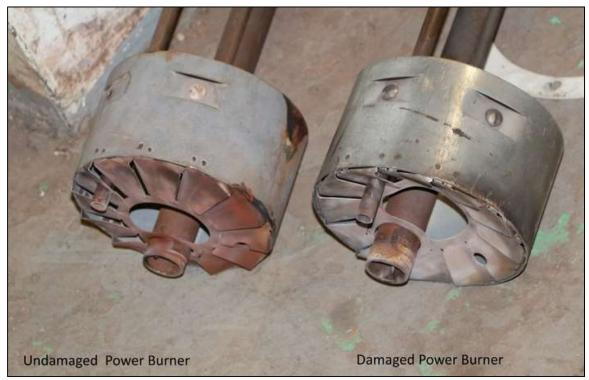
Photo 4: Undamaged power burner (exemplar) compared to damaged power burner. Diffuser deformed due to force of the explosion (fins flattened and pushed in).
