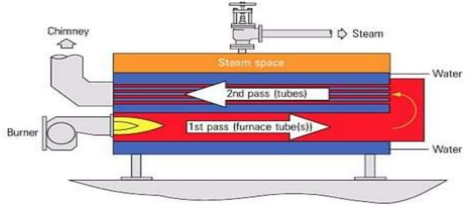
Diagram 1: A fire tube boiler
