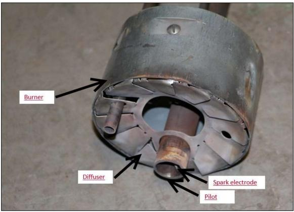
Photo 3: Power burner and its components.
