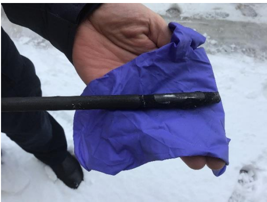
Photo #2: Heater element with dripping metal
