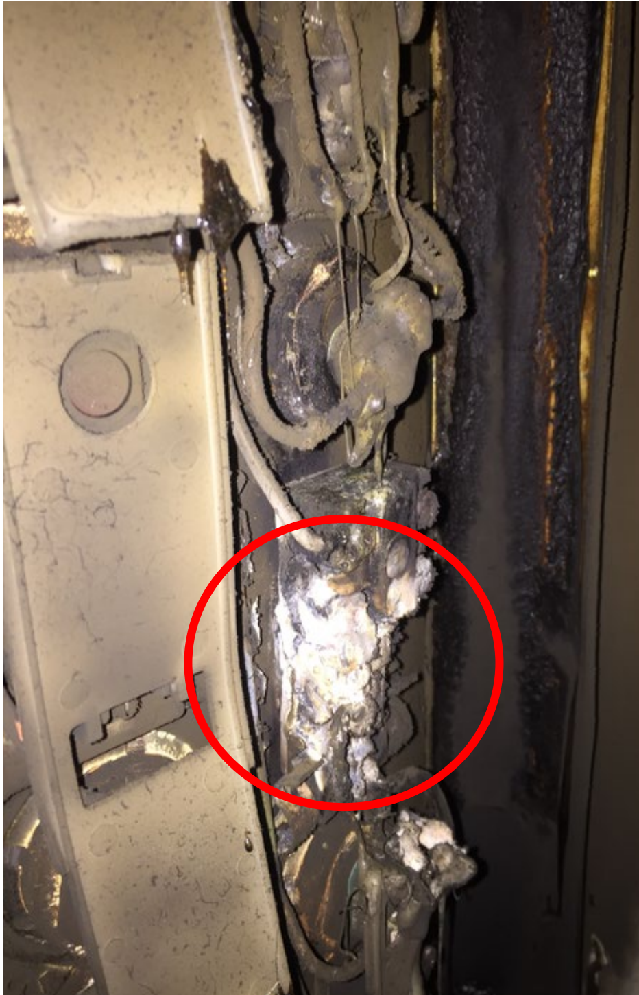
Photo 1 - Heating Element #2 point of origin damage
