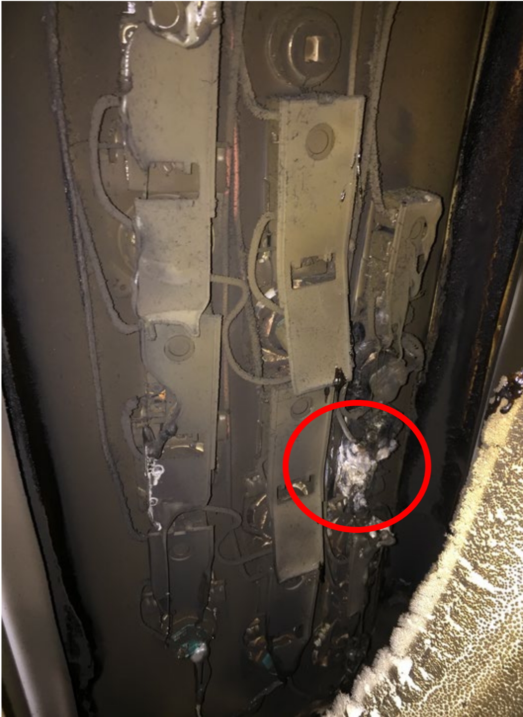
Photo 2 - Factor wired portion of HWT with majority of damage to middle heating element #2.
