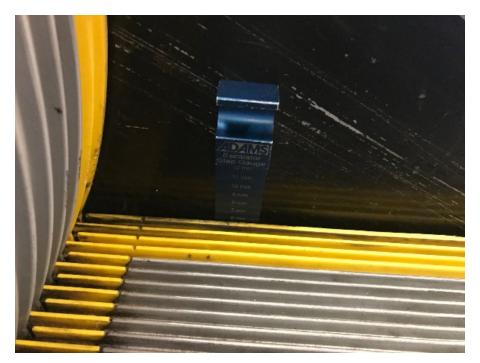
Picture 3 - Step skirt gap measurement at location where the shoe was caught
