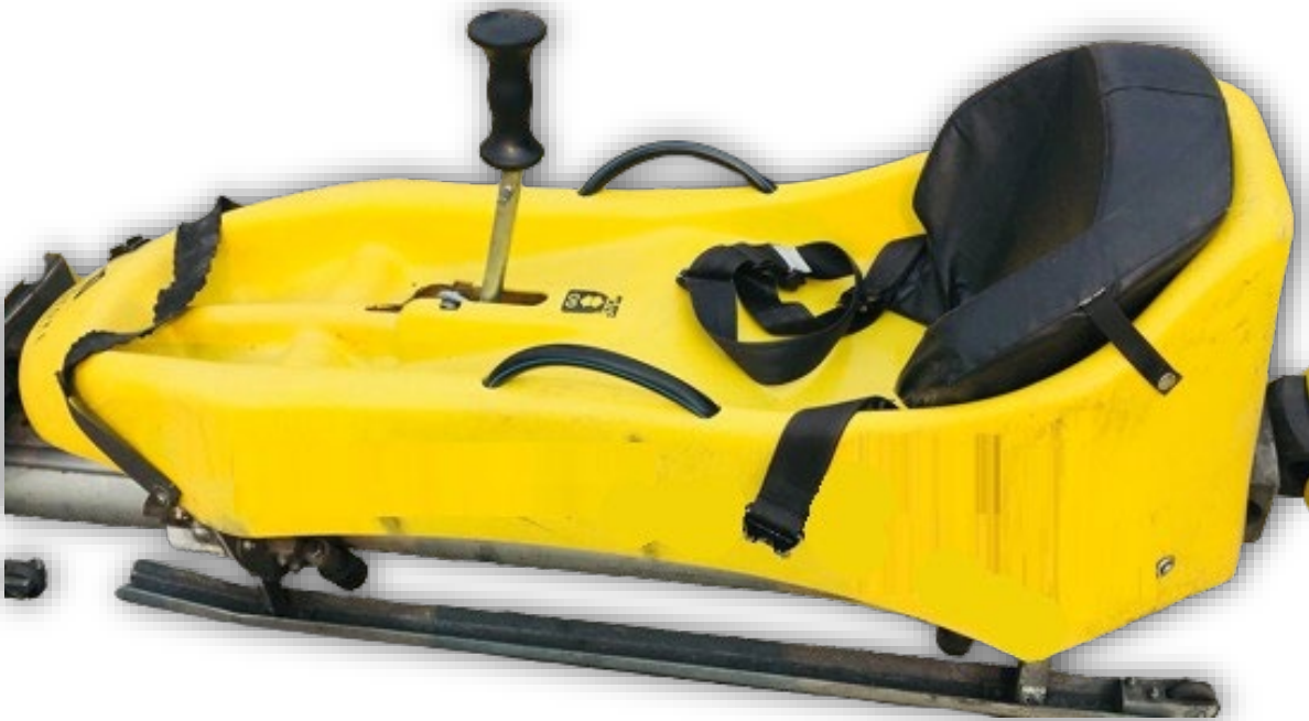
Image 5 – Seat showing no head rest (Below shows same manufacturer has design incorporating backrest.) Although backrest shown not every rider gets a backrest.
