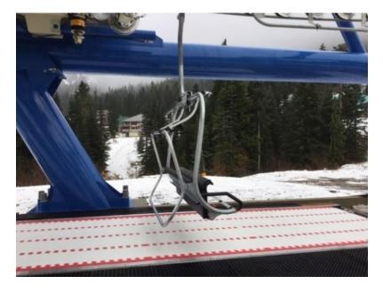
Chairlift loading area with carrier in place. Restraining bar is in the up position.
