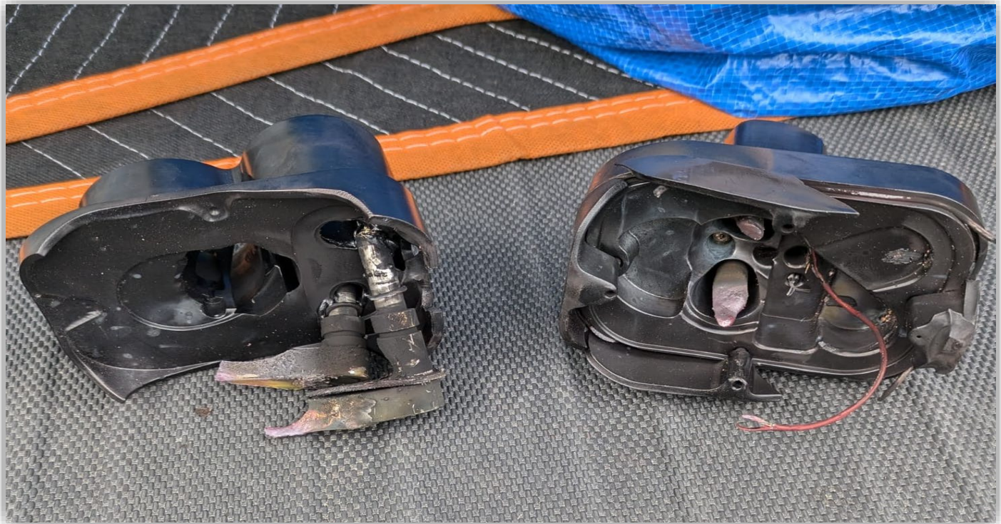
Image 2 - Adaptor blown in half with terminals showing signs of extreme heat.
