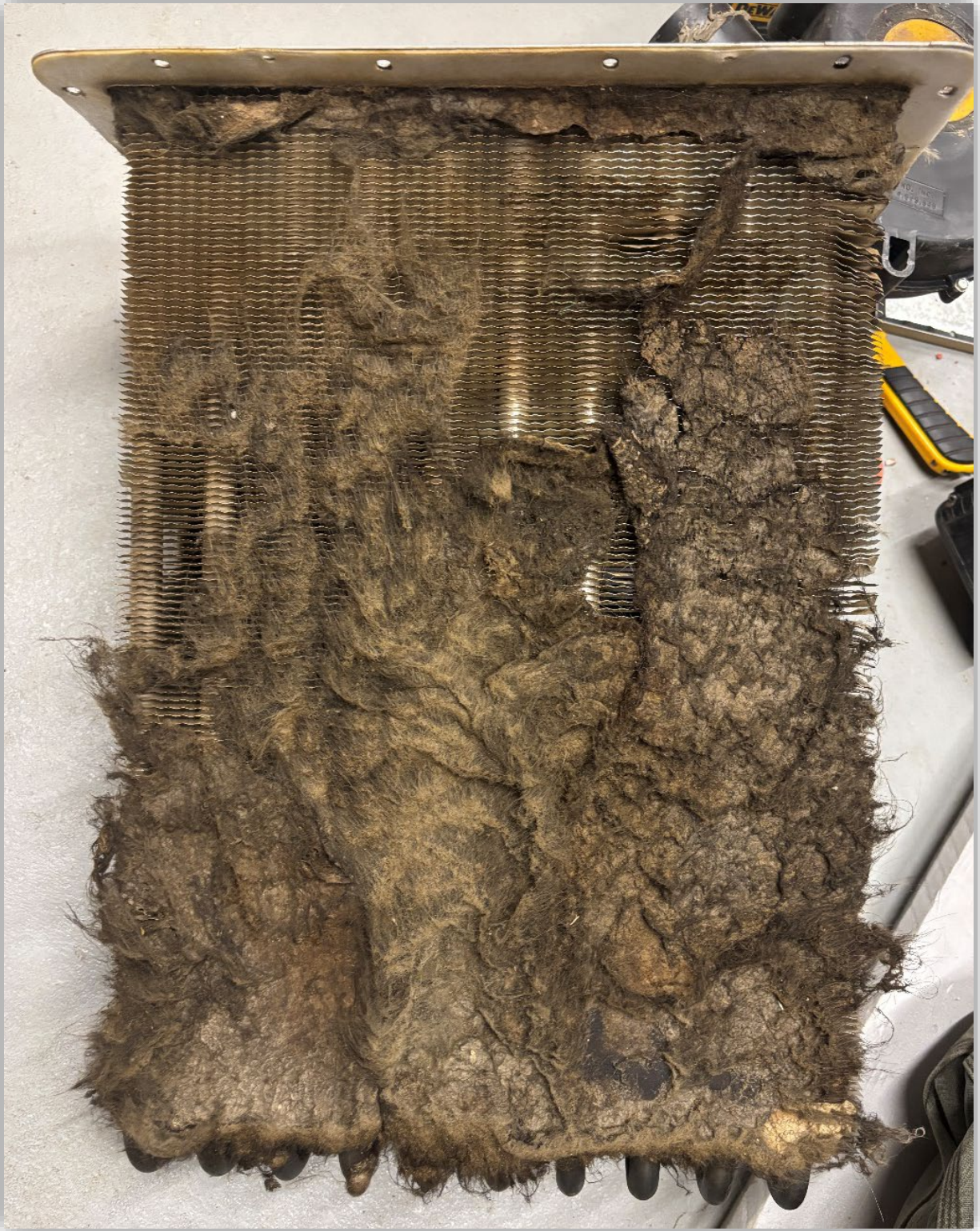
Image 8 – Dirty secondary heat exchanger found during furnace disassembly.
