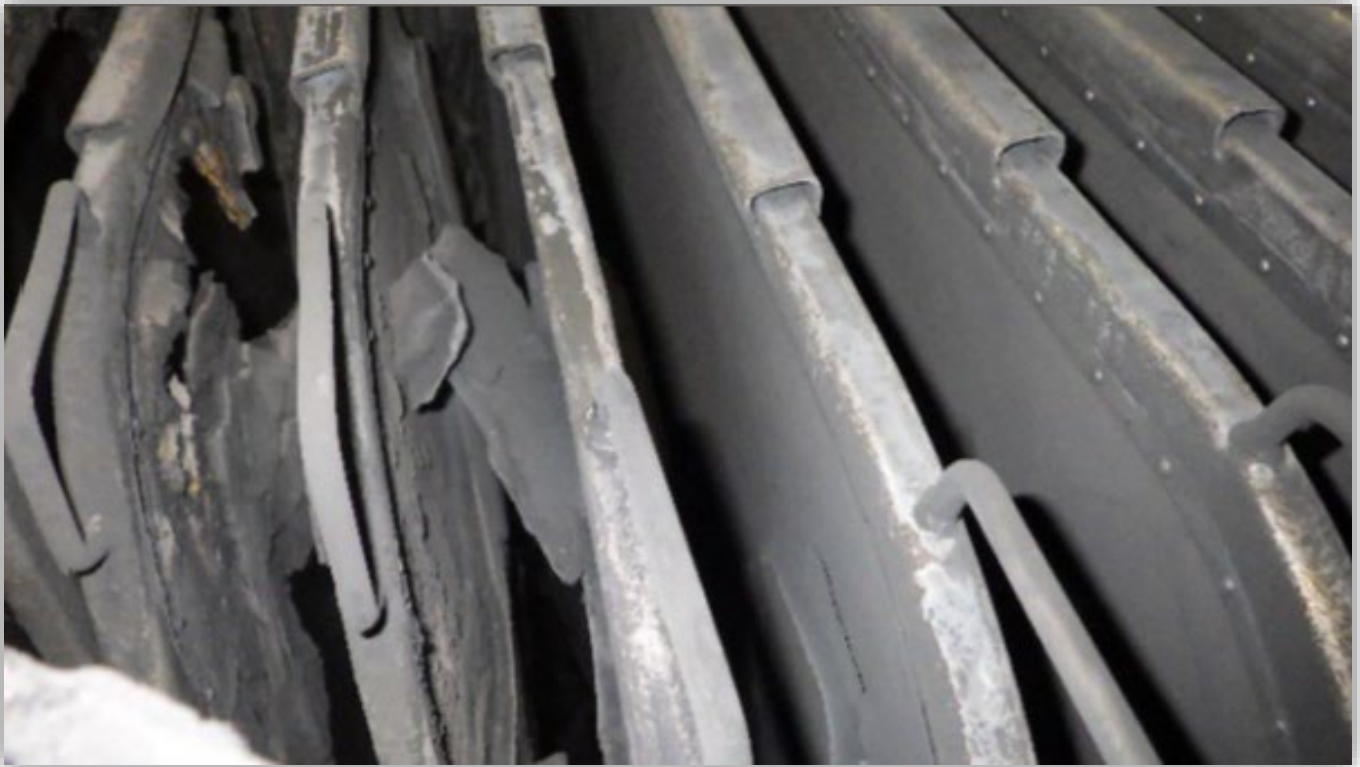
Image 3 - Damaged leaf filters.
