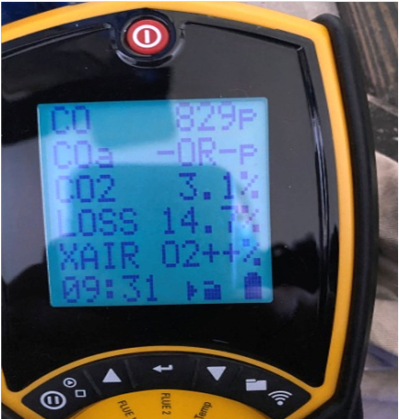
Photo 4 - CO reading (829ppm) at high fire as found setting with portable air conditioner on.
