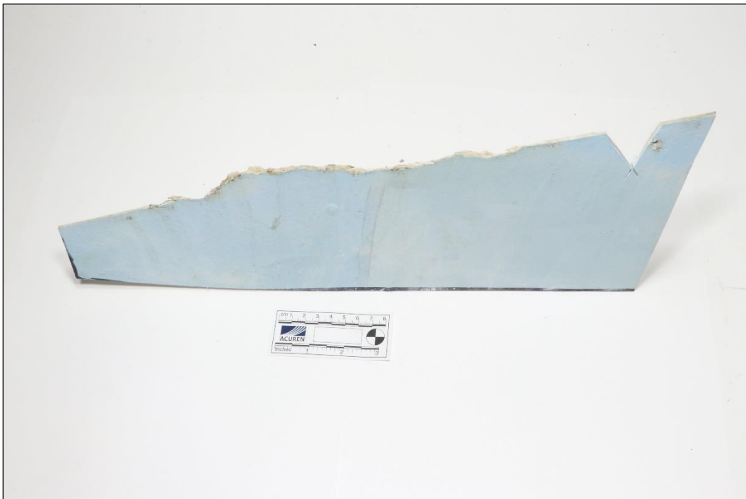
Figure 21 Sample I running surface. Notch was cut by others. Fracture is present along 80% of the top edge.
