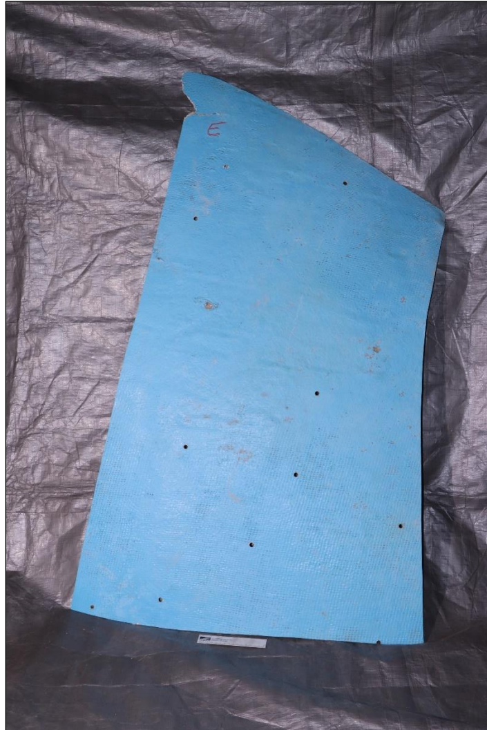
Figure 12 Sample E front surface. Note holes drilled for foam injection.
