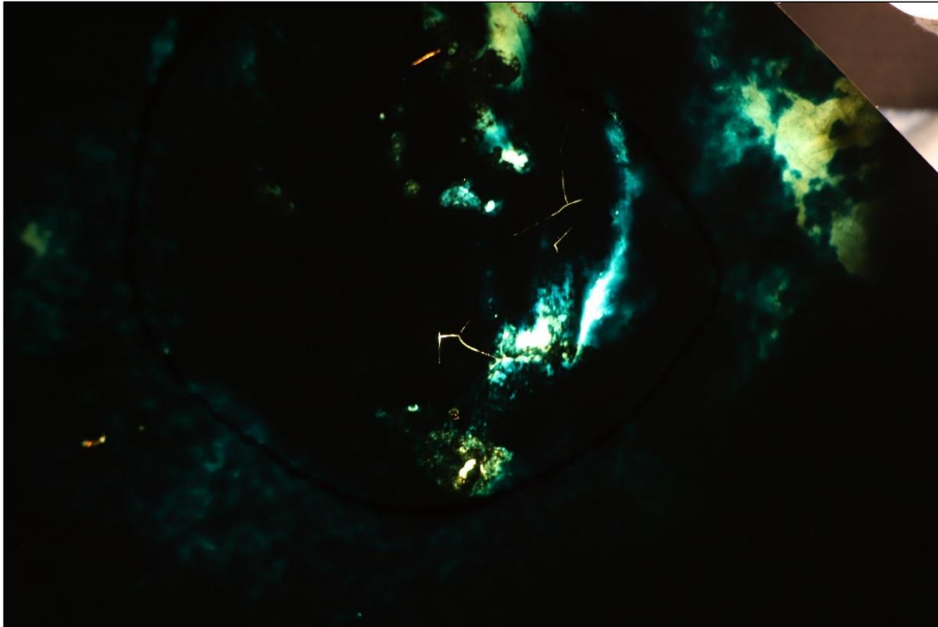
Figure 30 Cracking and weak areas exposed by backlighting sample B2.
