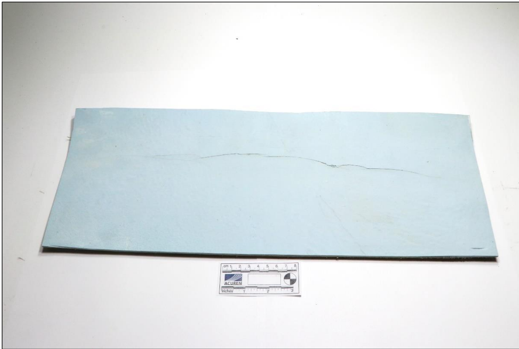
Figure 14 Sample F showing long transverse crack on running surface.
