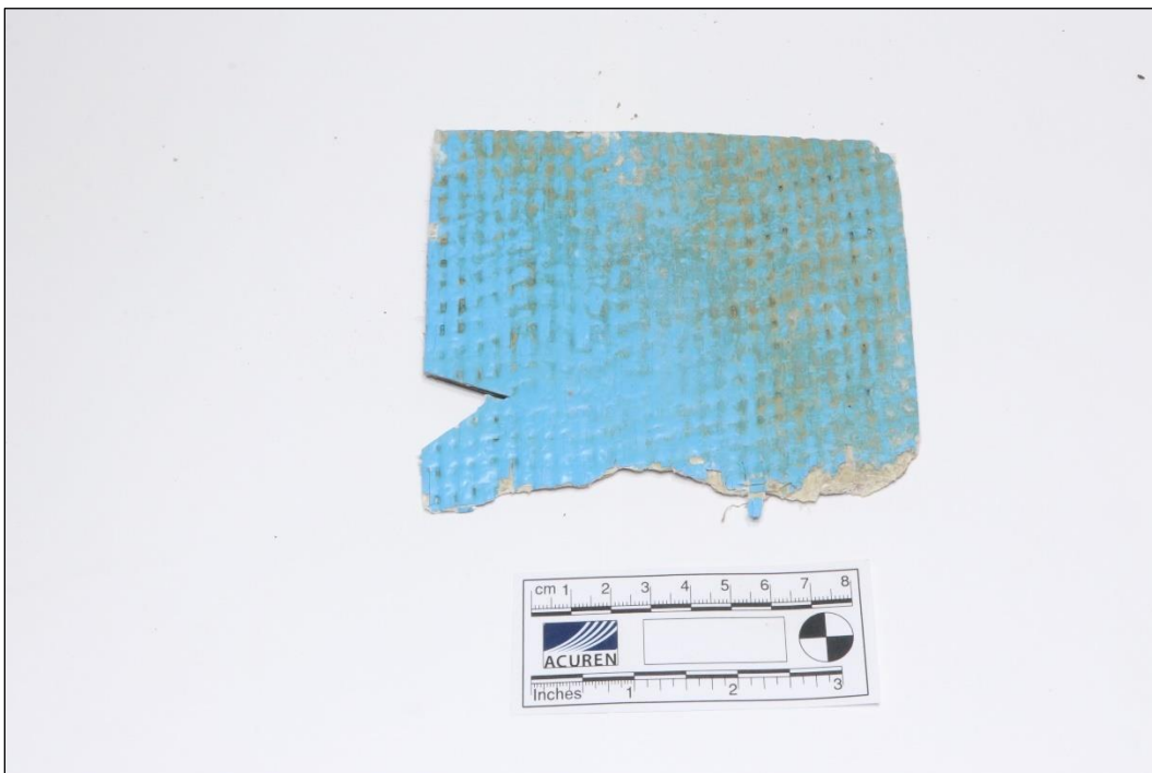
Figure 19 Sample H front surface containing fracture. Notch was cut by others.
