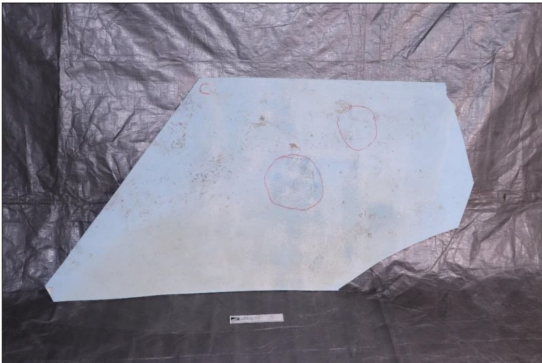
Figure 8 Sample C running surface showing discolouration and areas of surface damage.
