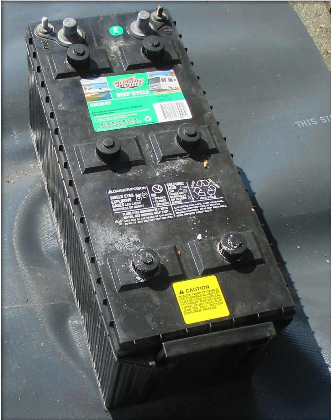
Figure 5 - Battery showing signs of electrolyte residue (white powder)
