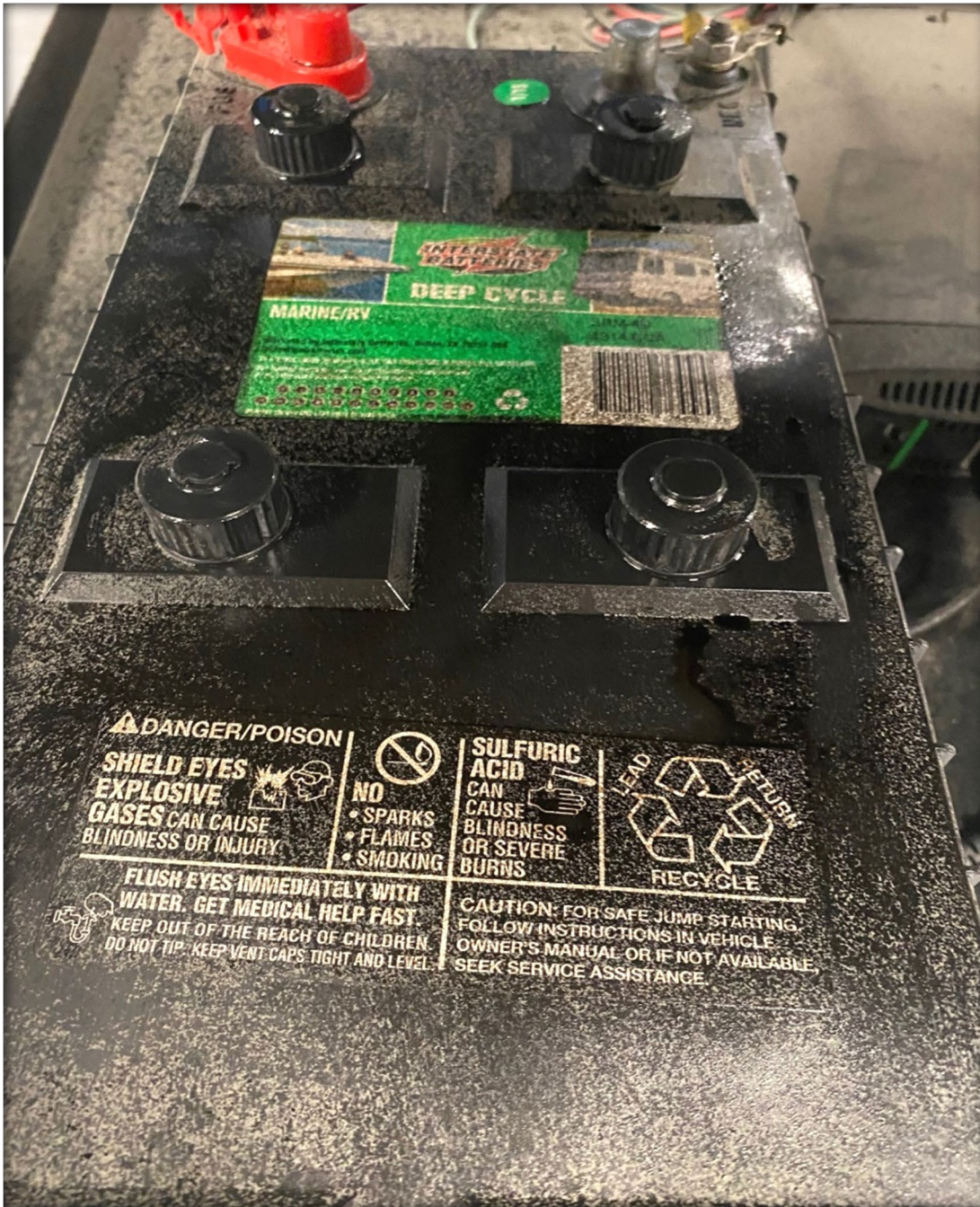
Figure 7 - Battery after the incident with fluid accumulations.
