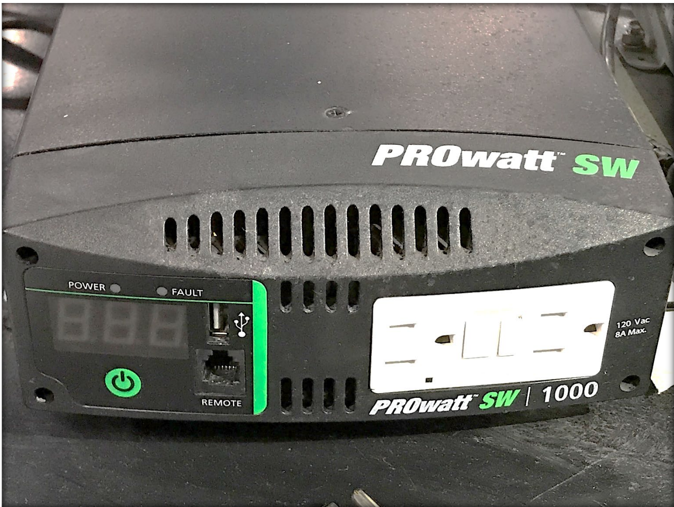
Figure 3 – Inverter that converts DC battery power to AC to power the Cubiscan 100
